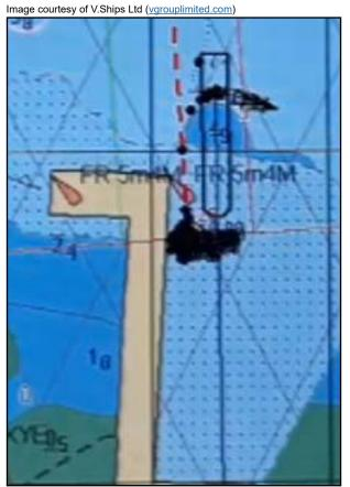
**Figure 4:** Screenshot of *Key Bora*'s ECDIS display as vessel grounded on the 4.9m hazard
