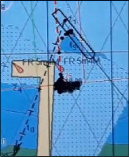
**Figure 14:** Screenshot from *Key Bora*'s ECDIS immediately prior to it grounding, predicting that it would strike the jetty
